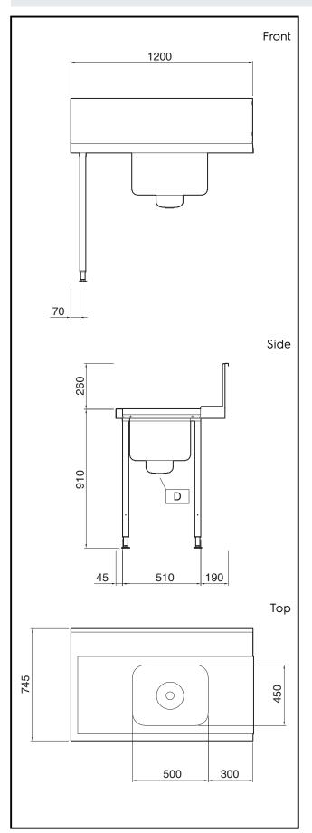
Handling System for Hood type Pre-wash Table with 500x400 Bowl and Strainer Left to Right, 1200mm
